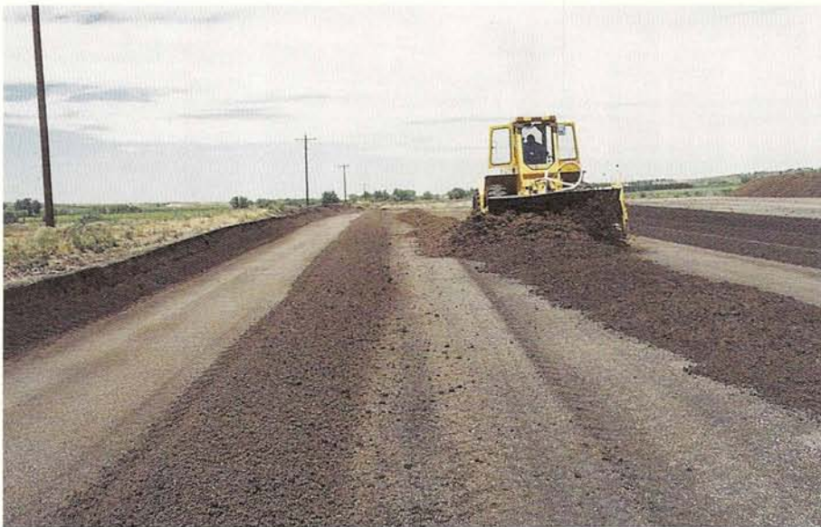
Blending cake biosolids in a 50/50 mix with previously composted biosolids.
